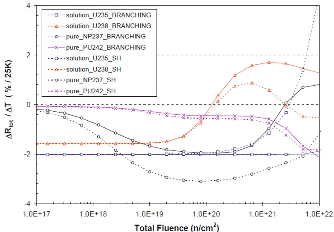
**Fig. 6.** Temperature dependence of the fission rates for different deposits. Branching cases show the difference in % between a reference irradiation case at 325 K and an instantaneous change in the temperature of +25 K. In the spectral history cases, we compare the nominal case at 325 K with a modified irradiation case at 350K.
