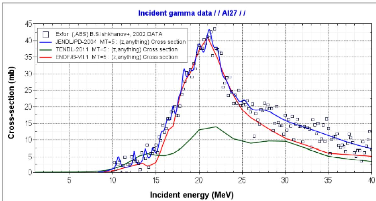
**Figure.** A comparison of total gamma cross section for Al27.
