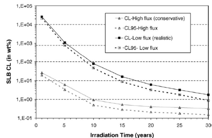
Fig. 1. Tungsten CL for SLB as function of irradiation time for two different neutron flux intensities. Uncertainties (CL95) are also provided
