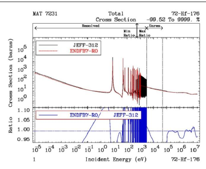
Figure 18. Total cross-section Hf-176
