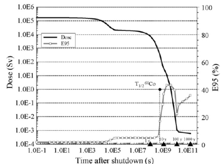
Fig. 1. Contact dose rate and relative error ( $E_{95}$ ) for the outboard DEMO blanket FW.
