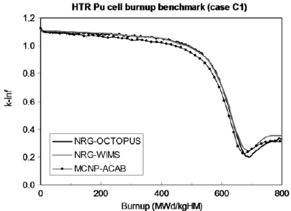
Fig. 5. Infinite multiplication factor as function of burn-up.
