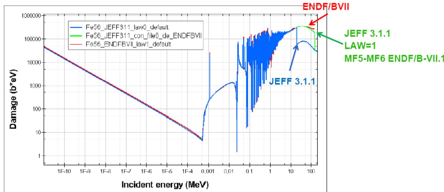
**Figure.** A comparison of Damage Energy Cross Section for Fe56.
